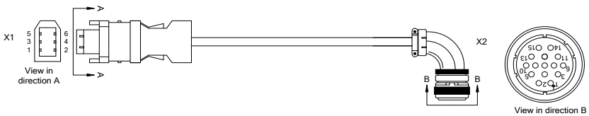
Figure 4-10 Absolute encoder motor wiring
